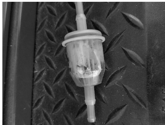
Fig. 4. Grass shavings visible inside fuel filter.
